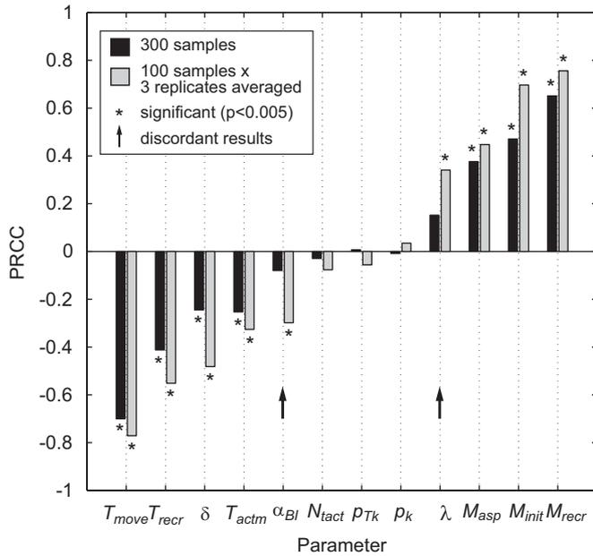
**Fig. 9.** Effect of aleatory uncertainty on LHS/PRCC and the benefit of averaging replicates. Model parameters were sampled 300 (black bars) or 100 times (gray bars). For the 100-sample condition, the three replicate model simulations were performed for each sample and averaged. Parameters with a PRCC significantly ( $p < 0.005$ ) different from zero are indicated with (\*). Parameters with discordant statistical significance between the two experimental conditions are indicated (arrow).
